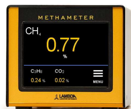
METHANMETER touch measures CH 4 concentration in the exit gas
